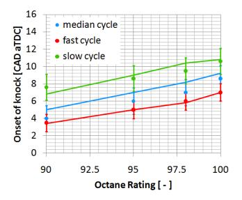
srm suite was used in *"blind test"* mode to simulate (solid lines in the above diagram) mean, fast and slow cycles including uncertainty for a range of automotive fuels. The model robustly predicted onset of knock with respect to experiments (represented by solid marks).
