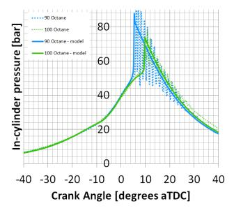
Above plots the in-cylinder pressure for 90 and 100 octane rated fuels. Experimental data was obtained from a manifold injection engine, engine speed 1500rpm, spark timing -20 CAD aTDC. The srm suite robustly computes heat release rates and the onset of knock.
