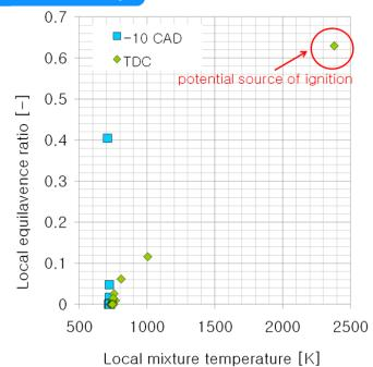
Corresponding in-cylinder local equivalence ratios and temperatures at 10 CAD bTDC and at TDC for a single oil droplet (here simulated as n-heptane). Results show that such a droplet could ignite forming a potential ignition source. This could "pre-ignite" the mixture prior to the spark, resulting in the mega knock cycle in the other graph
