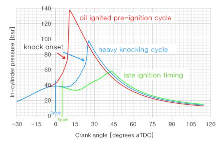
srm suite was used to simulate DISI combustion at high intake pressure (2.3bar). With an ignition timing of TDC, heavy knocking cycles were reported, however this was elevated by delaying the spark timing. Finally, an oil-ignited cycle was simulated – demonstrating similar characteristics to those observed in pre-ignition ("megaknock") combustion cycles.
