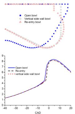
Adopted piston geometries and their impact on the in-cylinder pressure. Here the different geometries made only a subtle difference to the in-cylinder pressure profiles.
